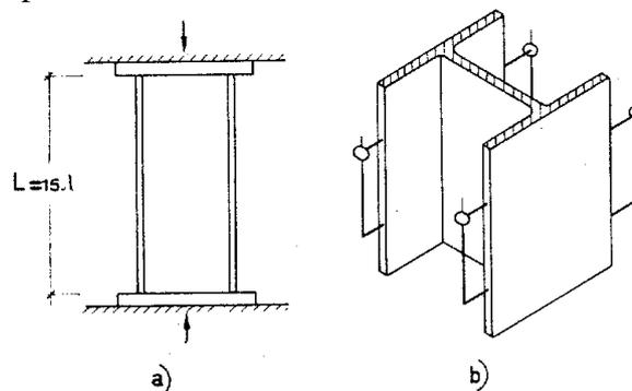
stub column test<sup>1</sup>
